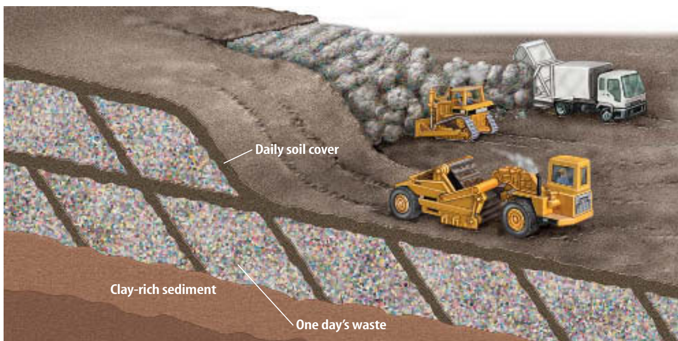
Figure 11 About 55 percent of the solid wastes collected in cities and towns is put in sanitary landfills. The landfills must be checked constantly for leaks so that the soil and the groundwater below it are not polluted.
