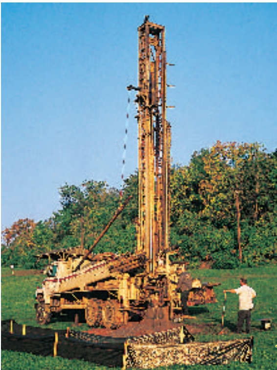
Figure 6 This truck has drilling equipment that can drill deep water wells in solid rock.
